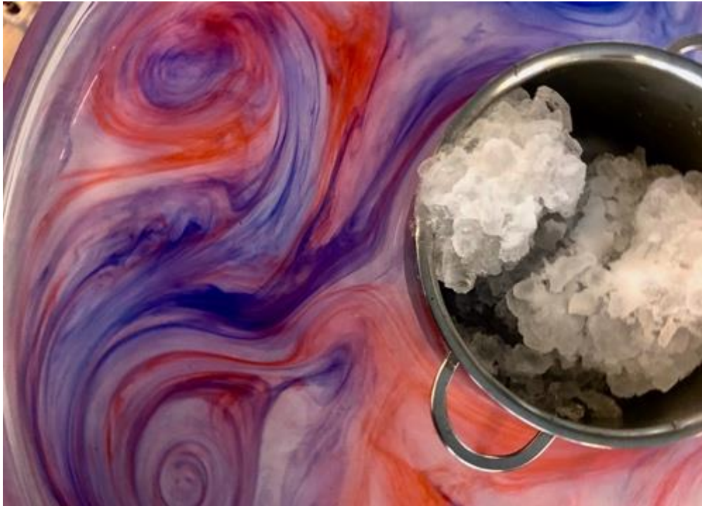
Rotating tank showing flow patterns. Photo: P. Reutter.
